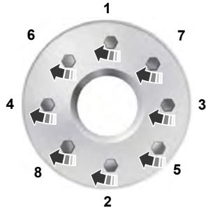
8-lug nut torque sequence
