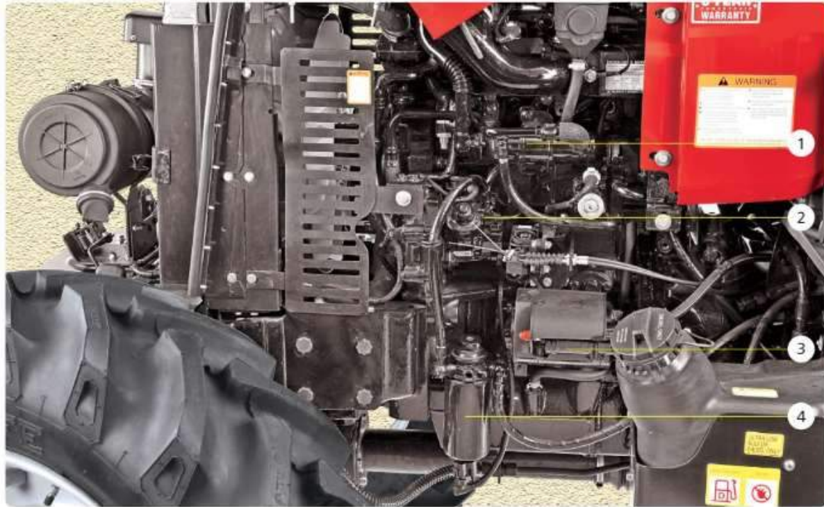
LH View : 1. EGR Cooler 2. Fuel Pump 3. Starter Motor 4. Fuel Filter
